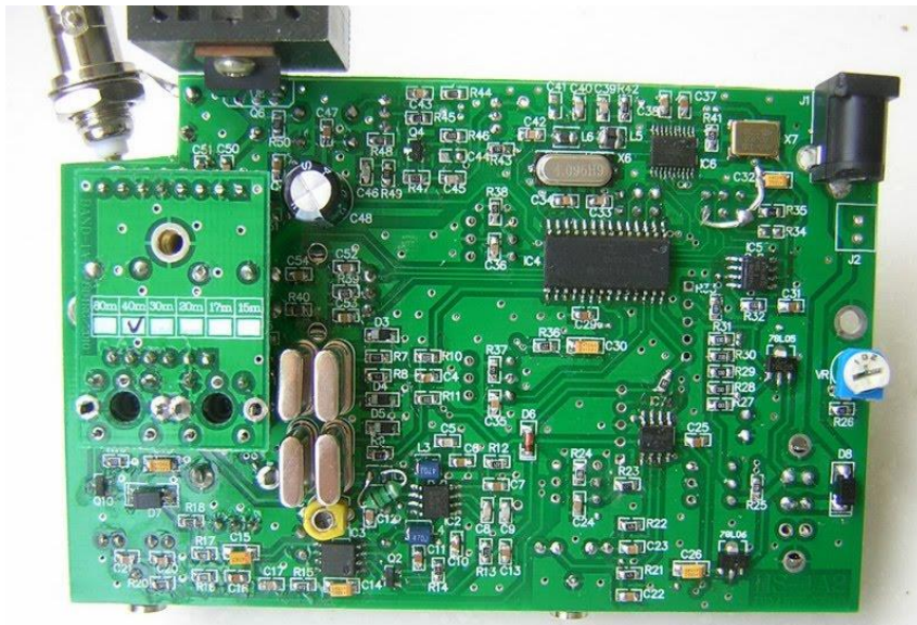
HS-1A main board – rear and front. D-9, the SWR diode is on the face of the board and is an axial version. The broadband transformer (T-1) feeding Q-10 is also found on the front of the board.
